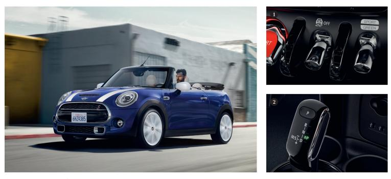
(1) MINI Driving Modes. (2) Electronic gear selector lever for 7-gear double-clutch transmission.
